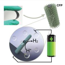
Nanostructured NiCo2O4/CuS heterostructure nanowires coated on a carbon fiber paper are fabricated as a self-standing 3D hydrogen evolution cathode. Benefitting from their structural merits including enhanced overall conductivity and rich effective active sites, this electrode shows exceptional high HER performance and excellent durability in acid medium, better than any noble metal free electrocatalyst reported to date.
